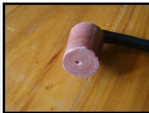
The angle joint fits into the top of the rubber stopper. You have to make a hole through the stopper. It only has to be a very small hole as seen here.
