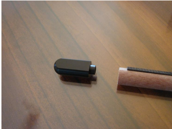
Press fit nose cone containing adjustable grub screw.
