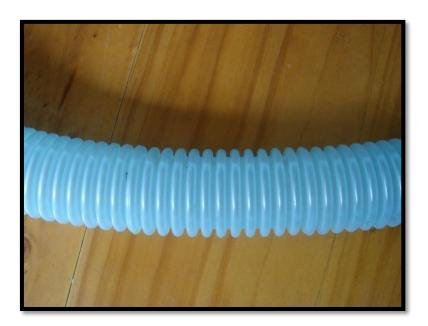
I glue a length of 19mm clear hose onto each end. This allows a good connection with a 19mm irrigation angle joint. You want one with a hose fitting on one side and a threaded end on the other. These fit into the bottom of most stocks. You might need a little Teflon tape or a bit of sanding for a good fit.
